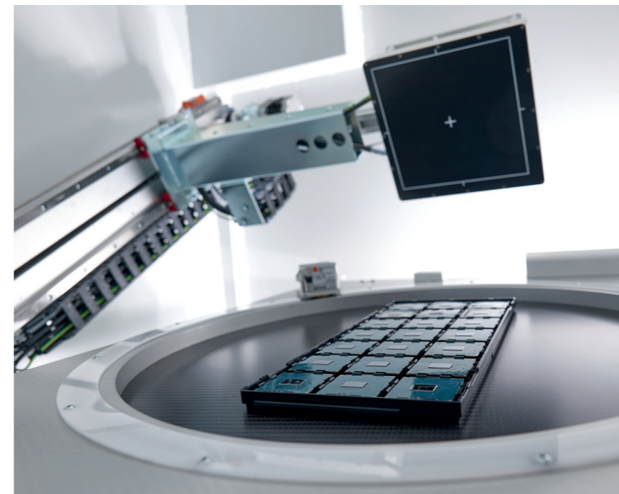
Automated 2D and laminography inspection for maximum productivity.
