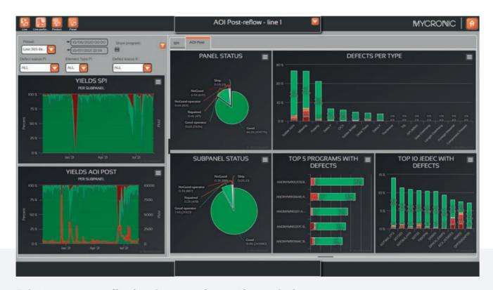
Print process quality has improved over the period but excessive warnings show we are operating close to process limits.
